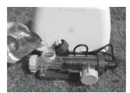
6. Open one side of the cell cover (11), drain and properly dispose of the vinegar. Connect the hose which goes from the pool to the cell. Flush the electrolytic cell housing with the pool water.
