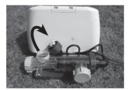
5. Pour kitchen grade vinegar into the electrolytic cell (9) to immerse the titanium electrodes. Soak for 1 hour.
