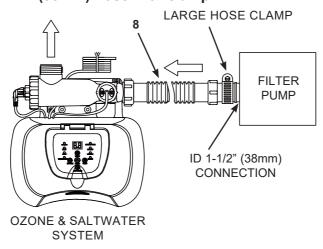
**1.** Connect the connector hose **(8)** to the filter pump outlet connection with a large hose clamp. Tighten securely.
