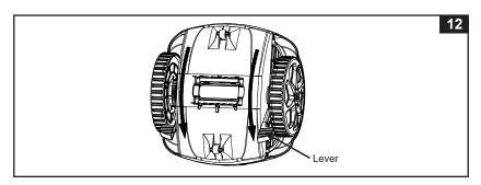
**6.** Remove the debris net **(2)** from the cleaner base **(3)**. If debris is on the debris net and cleaner base, use a garden hose to flush the debris off. See Fig. 13.
