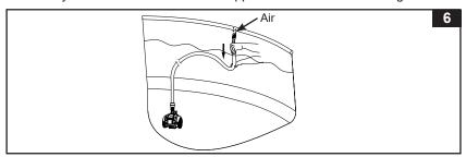
7. Once all the air has been released from the hose and the auto cleaner, attach the other end of the hose to the hose adaptor (4). See Fig. 7. When water begins flowing into the filter pump, open the air release valve on top of the filter pump cartridge chamber cover, lift and lower the pump hoses until water begins flowing out of the air release valve. Close the air release valve back. Refer to the filter pump manual for more details.
