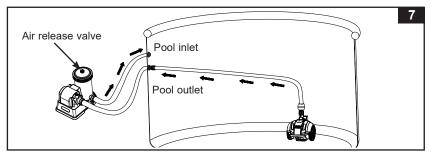
8. Turn on the filter pump. The auto cleaner is now moving and vacuuming the pool floor.
