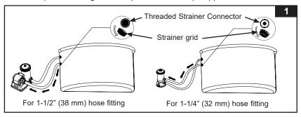
Screw the hose adaptor (4) to the threaded strainer connector, from inside of the pool. See Fig. 2.
