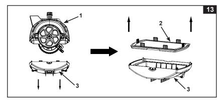
7. Reassemble auto cleaner debris net and base by reversing previous steps.
